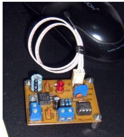
**Gambar 7.** Modul sensor temperatur LM35
